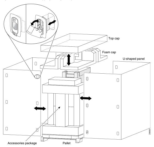
The accessories for the router ship in five boxes that are assembled into a package. (See Figure A-2.) The accessories package is packed against the back panel of the router on the extended deck of the pallet body.
